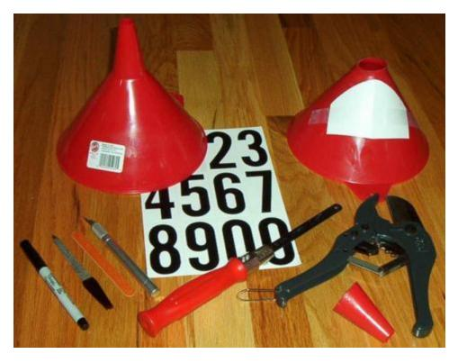
Oil/gas funnels with point cut off, slit cut, and number applied.
